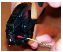
Figure 0-1 Crimp Tool for Ferrule
