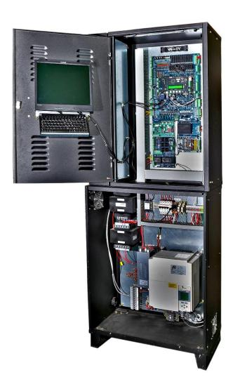
Figure 1-1: General Layout of the Controller
