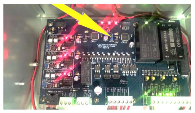
Figure 2-20: APS Selector Board Setup Jumper
